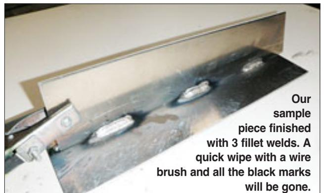
Our sample piece finished with 3 fillet welds. A quick wipe with a wire brush and all the black marks will be gone.
