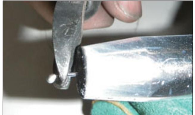
When the weld is finished, it is good practice to snip the end of the wire protruding from the MIG gun nozzle. After the welding operation, sometimes a ball appears at the end of the wire. To get a better weld start, you must remove this ball.
