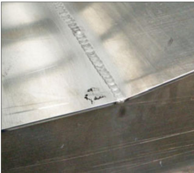
The finished welds require cleaning and external sanding if desired. After leak testing, commercial boats would be finished at this stage. On the inner chine weld we would remove the high spots, (stops and starts), and we may sand the external edge for visual appearance.
