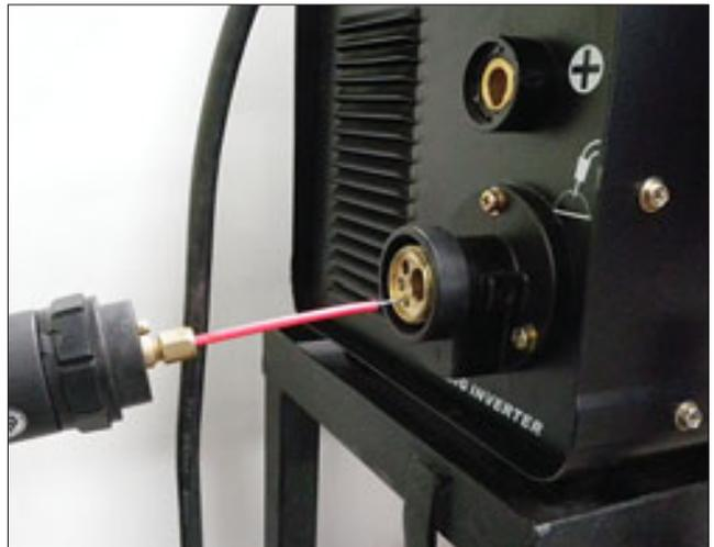
**Pic of Teflon liner at euro fitting end**
