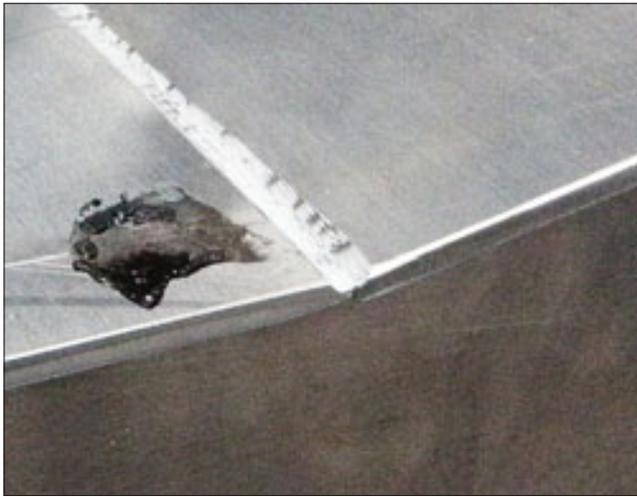
The picture above shows the corners prepared for the final weld.
