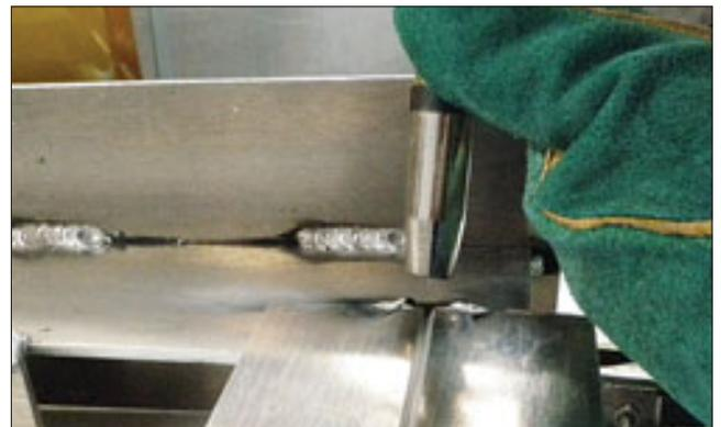
Side view showing the MIG gun angle when doing the butt weld.
