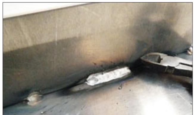
parts are intermittently stitched with a 50mm weld at 150mm spacing.
