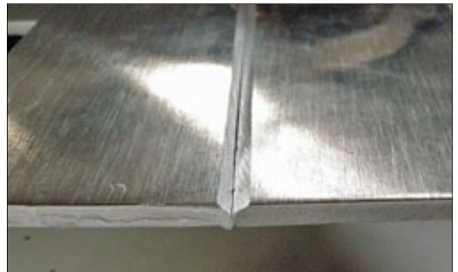
Close up view of edge preparation in readiness for butt weld. We will assume the plates are tacked on the back side for this example.
