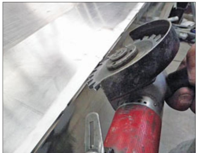
This photo shows the tool we use for back cutting. It is an air grinder with a metal cutting blade. These tools are excellent for removing large amounts of material quickly and without depositing grinding wheel material in the groove. These tools are also VERY dangerous and we would not recommend an inexperienced operator to use them.
