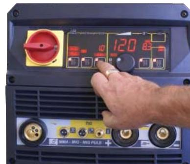
The Ergonomic and Auto Learning System is used in the powerful front panel interface where welding mode selection, program selection, adjustments and special settings coexist in a rugged panel, whereby a simple touch the user can instantly see the results they have selected.
