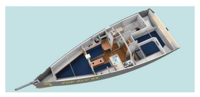
There is an aft cabin with double berth separated from the main ambient by a curtain, a double V berth forward and a comfortable saloon with 5 places, because one guest can seat in the forward bed, as we structured the mast frame in a way to obviate the need for a mast column, leaving the entrance to the forward cabin totally free.
