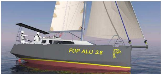
We fitted the Pop Alu 28 with an arch in the stern to receive two 140 Watt solar panels because we specify an electric outboard engine as main motorization option. With two 24 V lithium batteries and the solar panels, there is enough reserve for port manoeuvring.
